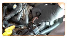
Disconnect the spark plug wires from the ignition coil.
