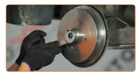
10 Remove the brake drum.
