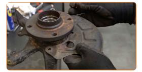
Screw in the fasteners of the brake disc cover. Use a combination spanner #10.
