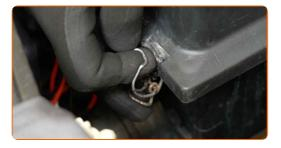
Screw in the fasteners of the air distribution housing assembly. Use a drive socket #7. Use a ratchet wrench.
