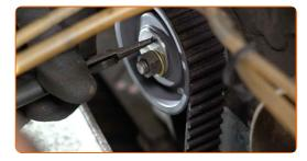
Remove the locking tool from the high pressure fuel pump pulley.
