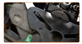
Remove the camshaft locking tool.
