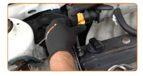
Remove the engine valve cover.
