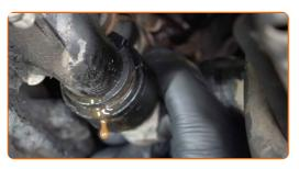
Drain the coolant from the engine.
