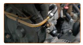
Unscrew the fasteners of the upper timing cover. Use a drive socket #13. Use a ratchet wrench.
