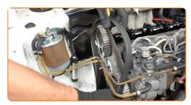
Loosen the vacuum pump pulley fastener. Use a universal pulley holder. Use a drive socket #19. Use a ratchet wrench.
