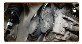
Clean the fastener of the crankshaft pulleys. Use a wire brush. Use WD-40 spray.
