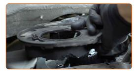
Turn the crankshaft gear. Use 12-point socket No.19. Use a ratchet wrench.
