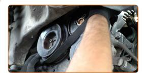
Replacement: water pump & timing belt kit – VW Caddy II Estate (9K9B).
