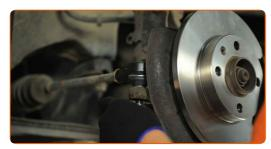
Tighten the fastening nut connecting the tie rod end to the steering knuckle. Use a drive socket #19. Use a torque wrench. Tighten it to 35 nm torque.
