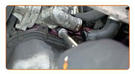
9 Remove the thermostat housing.
