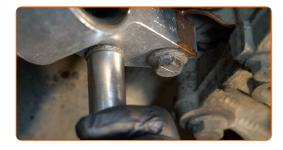
Screw the front arm fastener. Use a drive socket #18. Use a ratchet wrench.
