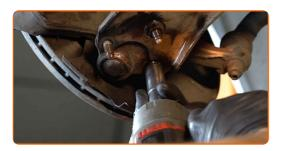
Unscrew the front arm fastener. Use a drive socket #18. Use a tap wrench.
