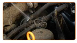
Loosen the fastening clamps of the fuel filter pipes. Use hose clamp pliers with retainer.
