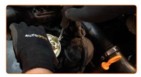
Remove the o-rings. Use a flat screwdriver.
