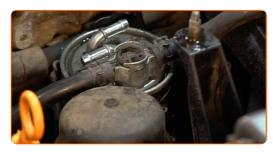
Disconnect the pipe from the fuel filter.
