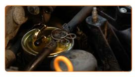
Attach the tubes to the fuel filter.
