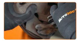
Detach the driveshaft from the steering knuckle.
