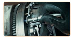
Align the clutch disc. Use a crowbar.
