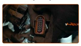
Detach the engine wiring harness.
