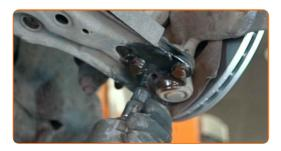
Disconnect the ball joint from the control arm.
