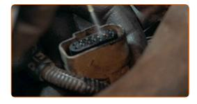
Connect the engine wiring harness connector.
