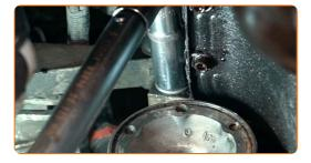
Attach the gear shift cable retaining clip.
