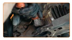
90 Install the steering knuckle on the CV axle.
