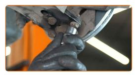
Attach the transmission sensor connector.
