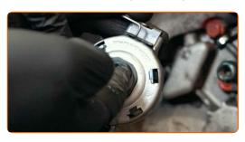
63 Install the new release bearing.
