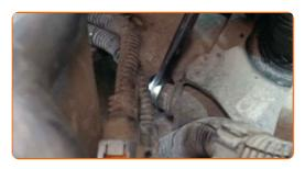
Remove the bottom gearbox mount. 46
