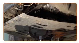
6.1 Clean the area around the gearbox housing filler hole.
