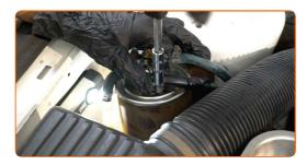
Screw in the fuel filter mounting bracket. Use a drive socket #13. Use a ratchet wrench.
