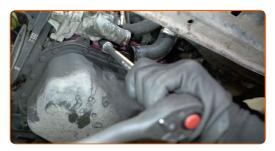
Remove the thermostat housing.
