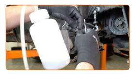
Undo the brake bleeder screw. Use a combination spanner #7.
