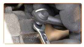
Press the brake pedal several times to remove any air from the system.
