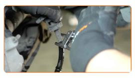
Unscrew the brake hose from the brake caliper.
