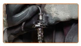
Remove the brake hose clamp.
