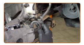
Clean the area where the brake hose is connected to the brake caliper and to the brake circuit pipe. Use a wire brush. Use WD-40 spray.
