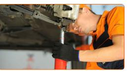
37 Fix the shock absorber strut on the steering knuckle. Use a hammer.
