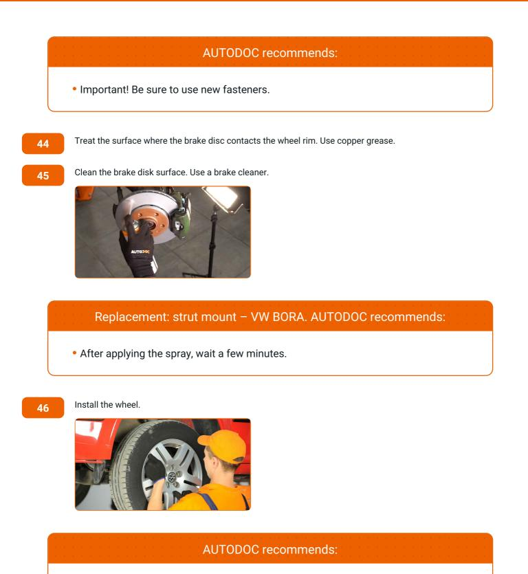
• Important! Hold the wheel while screwing in the fastening bolts. VW BORA
