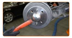
27 Treat the surface where the wheel rim contacts the brake drum. Use high-temperature ceramic grease.
