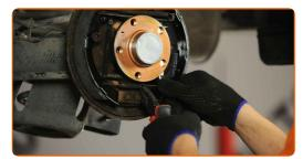
Insert retaining springs into pin slots. Use pliers.
