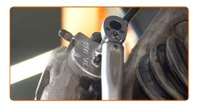
Remove the brake hose clamp.
