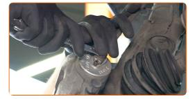
Loosen the fastener connecting the brake pipe to the brake hose. Use a combination spanner #11.
