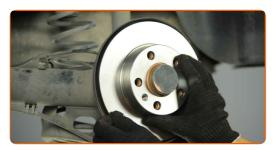
Tighten the brake disc fastening. Use a Phillips screwdriver. Use a torque wrench. Tighten it to 4 Nm torque.
