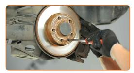
16 Remove the brake disc.
