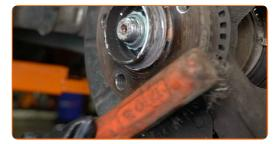
Treat the contacting surface. Use ceramic grease.
