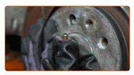
15 Remove the brake disc.
