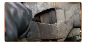
11 Remove the brake caliper.
