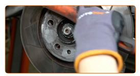
Unscrew the brake disc fasteners. Use an impact screwdriver. Use a hammer.
