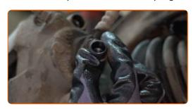
9 Unscrew the brake caliper fasteners. Use HEX No.H7. Use a ratchet wrench.
