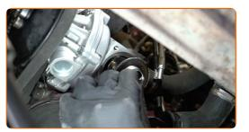
Replacement: engine thermostat – VW Bora Variant (1J6). Tip:
