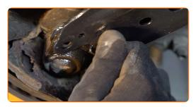
Screw the fasteners of the ball joint. Use a drive socket #13. Use a ratchet wrench.
