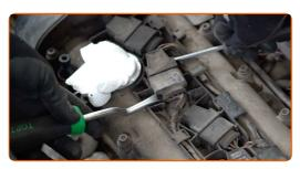
Undo the plastic locking tabs of the ignition coil connector. Use a flat screwdriver.
