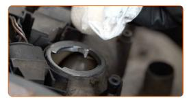
Install the oil filler neck. Screw in the oil filler neck.
