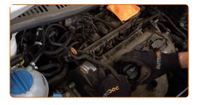
Unscrew the oil filler neck. Remove the oil filler neck.
