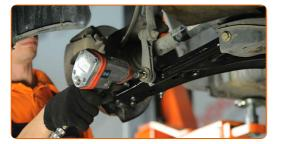
Mount the drive shaft into the wheel hub.
