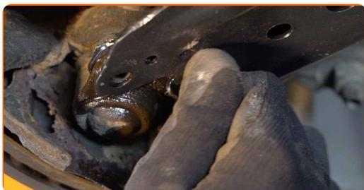
**20** Screw the fasteners of the ball joint. Use a drive socket #13. Use a ratchet wrench.
