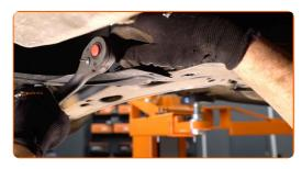
Remove the front fastener of the control arm.
