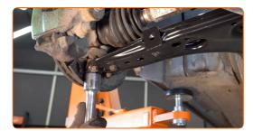
Tighten the front fastener connecting the control arm to the subframe. Use a drive socket #18. Use a torque wrench. Tighten it to 70 Nm torque.+90°
