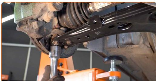
**22** Tighten the front fastener connecting the control arm to the subframe. Use a drive socket #18. Use a torque wrench. Tighten it to 70 Nm torque.+90°
