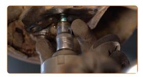
Loosen the front fastener of the control arm. Use a drive socket #18. Use a tap wrench.
