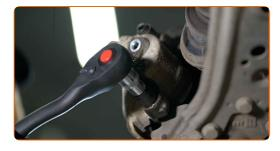
17 Remove the brake caliper.
