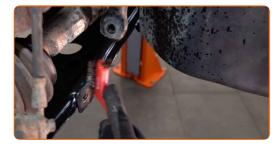
Install a new rod, tighten the fasteners.
