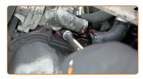
Remove the thermostat housing.
