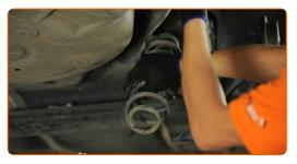
Remove the rubber spring spacer.
