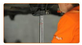
Tighten the lower fastener of the shock absorber. Use a combination spanner #16. Use a drive socket #16. Use a torque wrench. Tighten it to 40 Nm torque.+90°
