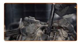
Take out the spark plugs. Use a telescoping magnet.
