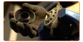
Clean the shock absorber rod fastener. Use a wire brush. Use WD-40 spray.
