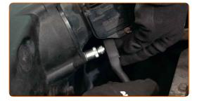
9 Remove the mass air flow sensor.
