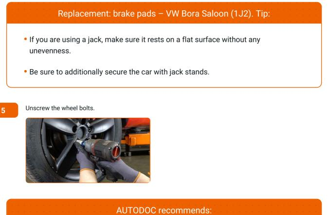
• Warning! To avoid injury, hold the wheel while unscrewing the fastening bolts. VW Bora Saloon (1J2)
