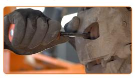
10 Remove the brake caliper.
