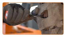
10 Remove the brake caliper.
