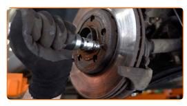
Remove the brake disc.
