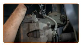
Unscrew the brake hose from the brake caliper. Use a combination spanner #11. Move the brake hose aside. Tie the brake hose to the car body with a hook or a piece of wire.
