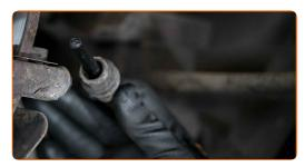
Clean old grease and rust stains, if there are any, from the caliper guide pins and guide pin boots. Use a brake cleaner.
