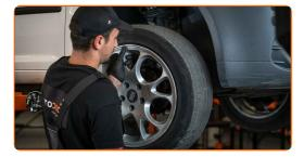
Turn the steering knuckle to the right to get access to the brake hose bolt and brake pad wear sensor.
