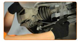
Loosen the fastener of the driveshaft. Use a drive socket #30. Use a ratchet wrench.
