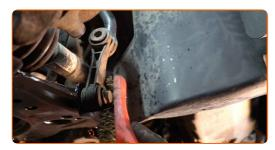
Unscrew the fastener connecting the stabilizer link to the stabilizer bar. Use a combination spanner #16. Use HEX No.H10. Use a ratchet wrench.
