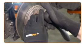
15 Remove the brake disc.
