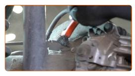
Detach the ABS sensor connector. Use a flat screwdriver.
