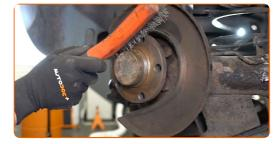
24 Install the brake disc.
