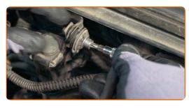
6 Unscrew the brake fluid reservoir cap.
