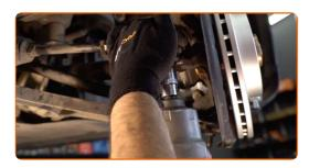
Tighten the fastening nut connecting the tie rod end to the steering knuckle. Use a drive socket #18. Use a torque 16 wrench. Tighten it to 20 Nm torque.+90°
