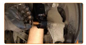
Support the stub axle. Use a hydraulic transmission jack.
