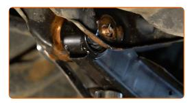
Remove the support from under the arm.
