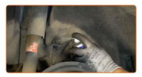
Unscrew the wheel arch cover fasteners. Use Torx T25. Use a ratchet wrench.
