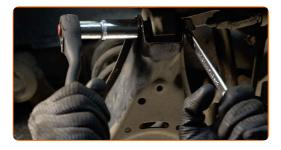
Remove the fastening bolt. Use a crowbar.
