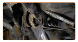
Remove the support from under the arm.
