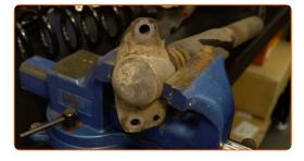
Remove the protective cap of the shock absorber mount. Use a crowbar.
