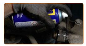
Unscrew the lower fasteners of the shock absorber. Use a drive socket #21. Use a ratchet wrench.
