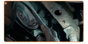
Replacement: serpentine belt – VW Beetle Hatchback (5C1, 5C2). Tip:
