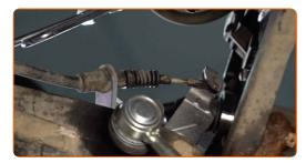
Unscrew the brake hose plug. Use HEX No.H7. Use a ratchet wrench.
