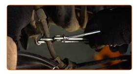
Remove the brake hose clamp.
