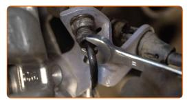
Treat the brake hose. Treat the brake pipe. Use a brake cleaner.
