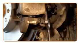
18 Remove the brake caliper.
