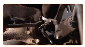
Remove the retaining clip of the parking brake cable. Use a crowbar.
