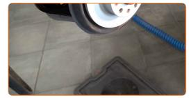
Unscrew the fastener connecting the brake pipe to the brake hose. Use a combination spanner #11.
