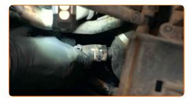
Attach the clamp of the upper coolant hose. Use clic-R collar pliers.
