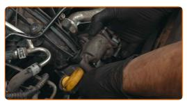
Tighten the throttle body fasteners to the air intake manifold. Use Torx T27. Use a torque wrench. Tighten it to 14 nm torque.
