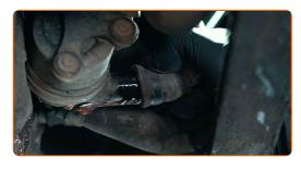
Drain the coolant from the engine.
