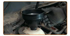
Pour coolant in the coolant reservoir.
