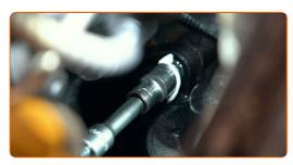
Tighten the thermostat housing fasteners. Use a drive socket #10. Use a torque wrench. Tighten it to 9 nm torque.
