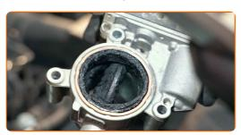
Replacement: engine thermostat – VW Beetle Convertible (5C7, 5C8).
