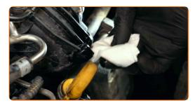
Install the throttle valve on the intake manifold. Install the fastening bolts.
