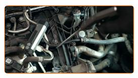
Disconnect the throttle body connector.
