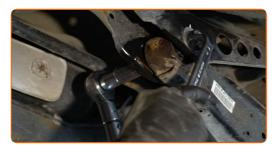
Remove the support from under the arm.
