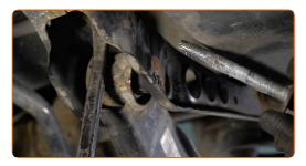
Remove the support from under the arm.
