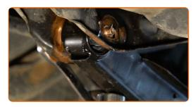
Remove the support from under the arm.
