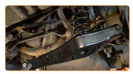
Install the fastening bolt. Use a crowbar.
