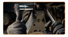
Remove the fastening bolt. Use a crowbar.
