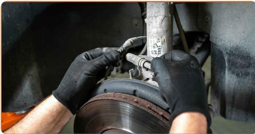
21 Clean the fasteners connecting the stabiliser link to the shock strut, and those connecting the shock strut to the steering knuckle. Use a wire brush. Use WD-40 spray.
