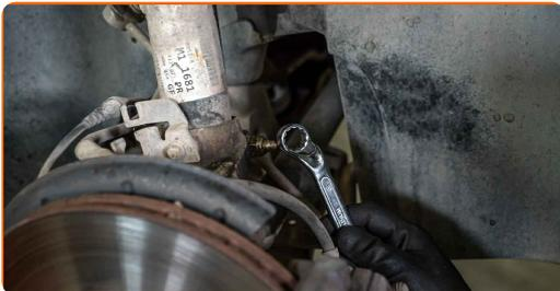
**25** Prop up the steering knuckle. Use a hydraulic transmission jack.
