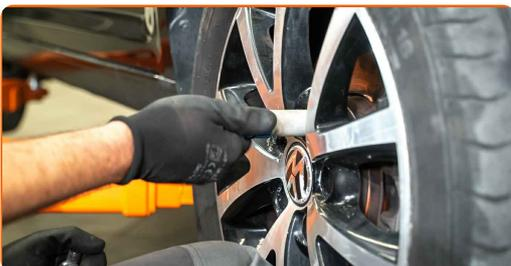
16 Loosen the wheel hub bolt. Use 15/16" drive 12-point socket.
