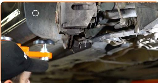
53 Install and tighten a new bolt of the steering knuckle. Important! Be sure to use new fasteners. Use a combination spanner #18. Use XZN #14. Use a drive socket #18. Use a torque wrench. Tighten it to 70 Nm torque.+90°
