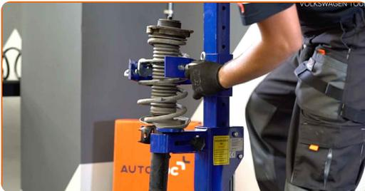
**34** Remove the strut rod nut. Use a combination spanner #18. Use HEX No.H6.
