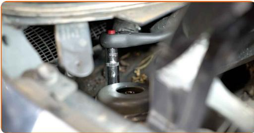
49 Fix the shock absorber strut on the steering knuckle.
