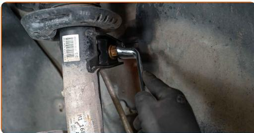
23 Remove the level control system sensor from the suspension control arm.
