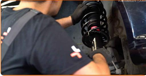
48 Tighten the shock strut top mount. Use a drive socket #13. Use a ratchet wrench.
