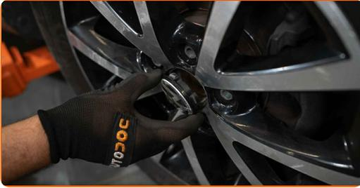
62 Lower the car and working in a cross order, tighten the wheel bolts. Use a torque wrench. Tighten it to 120 Nm torque.
