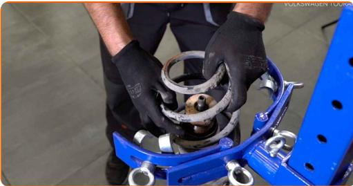
38 Remove the old shock absorber from the hydraulic coil spring compressor.
