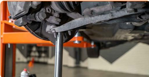
**26** Disconnect the steering knuckle from the shock absorber strut. Use a flat metal-working chisel. Use a hammer.
