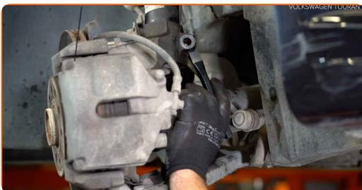
**27** Unscrew the fastener connecting the drive shaft to the wheel hub. Use 15/16" drive 12-point socket. Use a tap wrench.
