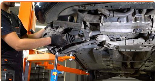
51 Attach the ball joint to the control arm.
