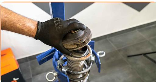
36 Release the coil spring.
