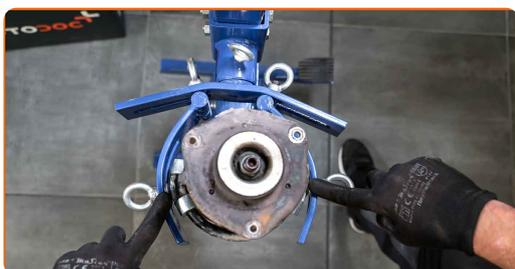
Replacement: suspension strut – VW Beetle Convertible (5C7, 5C8). Tip from AUTODOC experts:
