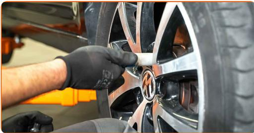
60 Tighten the bolt connecting the drive shaft to the wheel hub. Important! Be sure to use new fasteners. Use 15/16" drive 12-point socket. Use a torque wrench. Tighten it to 70 Nm torque.+90°
