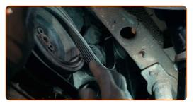
Replacement: serpentine belt – VW Beetle Convertible (5C7, 5C8). Tip:
