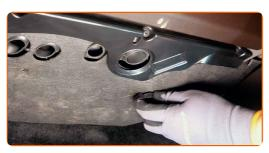
Remove the bottom cover of the glove box.
