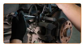
10 Remove the brake caliper.
