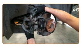
Replacement: brake pads – VW Beetle Convertible (5C7, 5C8). Professionals recommend:
