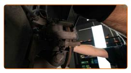
Unscrew the brake caliper fastening. Use a combination spanner #12. Use a combination spanner #19. Retain the guide pin with another spanner.
